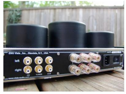
power tubes in conjunction with two ECC83/12AX7 signal tubes. Not only do these tubes sound great together – but they are easy to find and inexpensive to replace, making it perfectly ideal for tube swapping. Designed with ease of use and low maintenance in mind, the i84 is self biasing. Forget about having to take out the voltmeter and match each pot within tight tolerances every time you want to swap output tubes – that's already taken care of. You can literally just plug and play.
