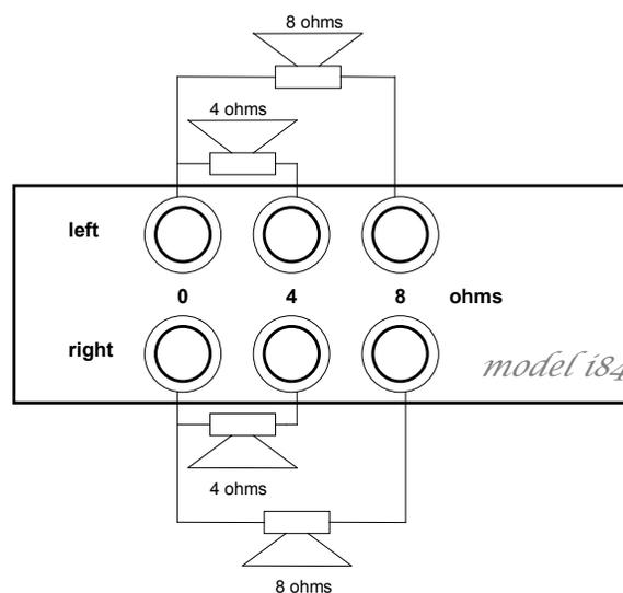
Figure 2: *model i84* speakers connection
