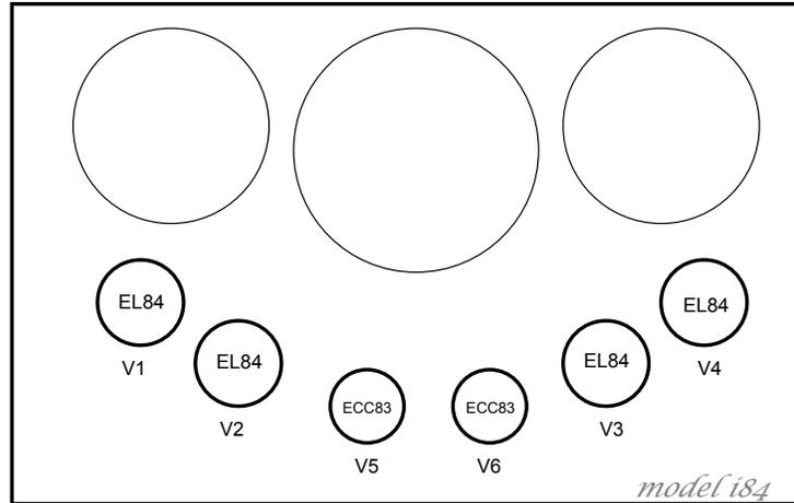
Figure 1: *model i84* tube layout
